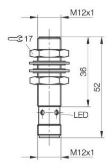
**Inductive Sensors** BES M12MF1-PSC30A-S04G-W M12x1 x 52 normally-open Sn=3mm shielded Factor 1
